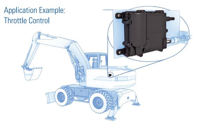
Throttle actuators allow automatic control of engine speed for reduced noise and emissions, and improved fuel economy.
