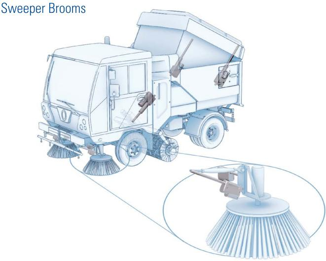
Actuators replace hydraulic and pneumatic cylinders for better controllability, smaller installations and eliminating the need of maintenance.
