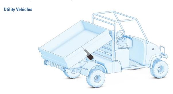
Electric linear actuators provide the rugged, efficiently controlled performance required by garden, construction and service vehicles.
