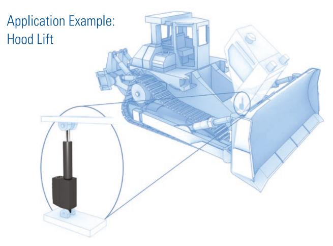
Hood lift actuators provide easy and safe access to engines for maintenance and repair work.
