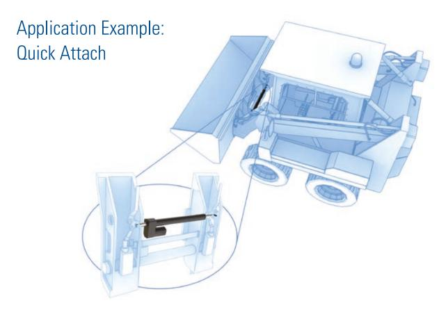
Quick-attach actuators allow the operator to change implements on the loader or skid steer without leaving the seat for improved productivity and safety.
