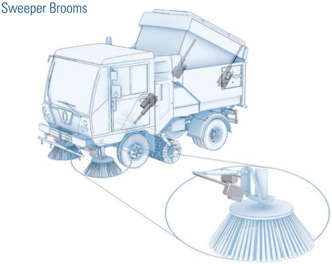
Actuators replace hydraulic and pneumatic cylinders for better controllability, smaller installations and eliminating the need of maintenance.
