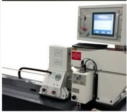
A dedicated lead-accuracy measurement device for miniature screws designed by Thomson can dynamically measure the full travel length of the screw and grade the accuracy per international standards.
