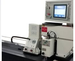
A dedicated lead accuracy measurement device for miniature screws designed by Thomson can dynamically measure the full travel length of the screw and grade the accuracy per international standards.
