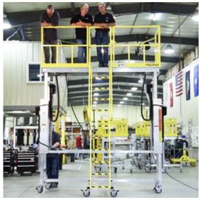
"Especially in comparison to hydraulic systems, the Thomson synchronised actuators provide us an optimal solution for our applications," said Spika. "With Thomson's synchronised actuators, our platforms stay level regardless of the load distribution; something that hydraulics cannot do easily."
